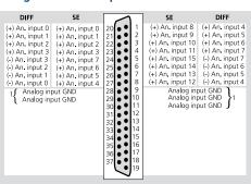
1: The analog inputs have a common ground line
