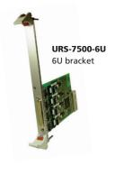
The setup of this serial communication board is determined by MX modules, which the board detects automatically. The serial interfaces can be configured with the following modes: RS232, RS422, RS485 and 20 mA Current Loop (with optical isolation).
